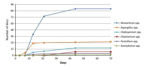
Fig. 2 Time (days) until first appearance of fungal growth/sporulation on disks (both face and reverse) from panels 10-13 (n = 96).
